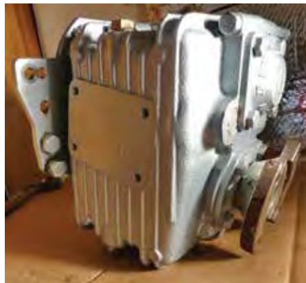
The ZF 15MA transmission showing the two port side bolts that remain on it
