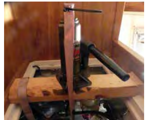
The bottle jack on the 2x4 that was held in place so it would not move
