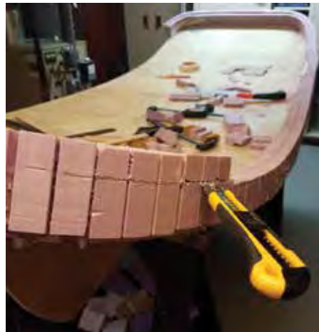
Two layers of Styrofoam were epoxied to the outside and forward edges of the plywood and carved into a flared lip.
