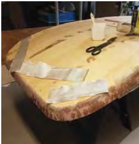
The tight corners around the flared lip were the most difficult areas to fiberglass.
