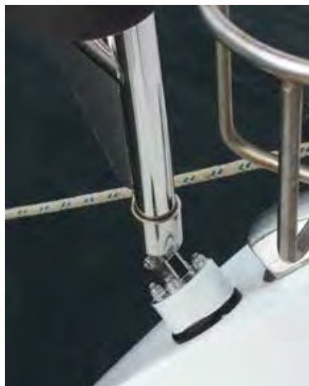
Fabricated Davit Base Spacer (wrapped with rigging tape)
