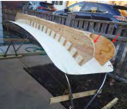
The dodger takes shape with the plywood core bent and attached to the bending frame (see red arrows) and then set on the stainless steel tubing to confirm its shape and fit.
