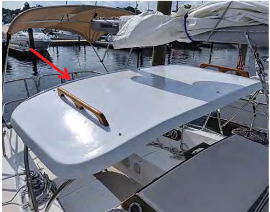
End Result. Red arrow indicates the rain guard.
