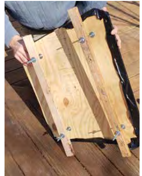
A view of the underside of the temporary hatchcover and the two attachment bars and bolts used to hold the temporary hatch in place below the foredeck.
