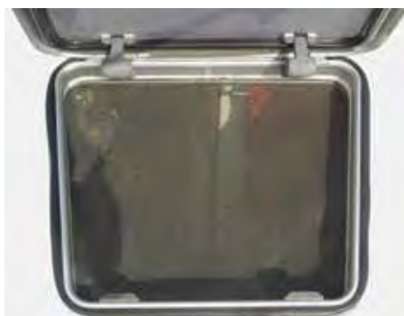
Forward deck hatch and added rubber gasket
