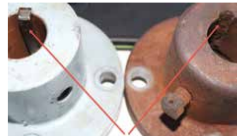
Image of new and old shaft coupler, arrows point to sheered key
