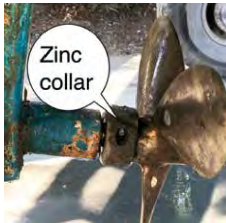
Zinc collar positioned too close to cutlass bearing
