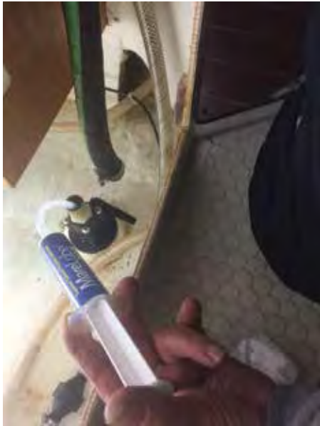
Picture 5: Then I used the MareLube Reach tool that comes preloaded with grease to lubricate from above and below all of the other seacocks to make sure I do not have to do this again. The package says it contains enough grease to lube 20 seacocks.
