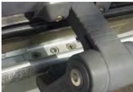
Forward deck hatch hinge and mounting screws
