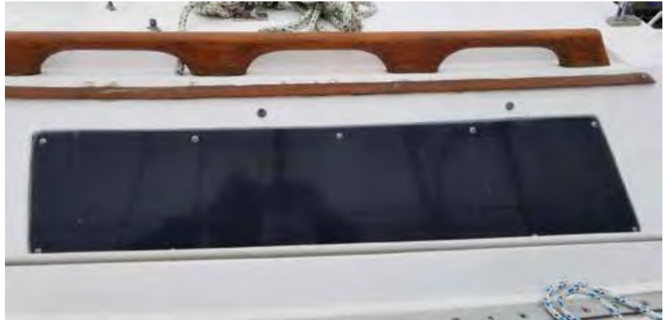
Original 30 year old windows on Afternoon delight, leaking and crazed
