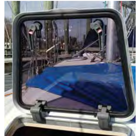
Newly installed Lewmar Ocean 65 hatch cover with its new crystal clear acrylic lens
