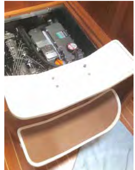
Showing the adhesive pad removed prior to temporary removal of the second tread.
