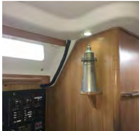
Aft overhead area near navigation station showing new line conduit in corner.
