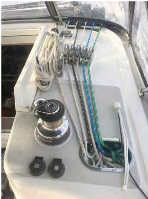
Starboard companionway deck with electrical feed-through in place.
