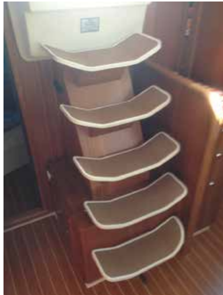
The companionway stair assembly. Note the position of the piano hinge
