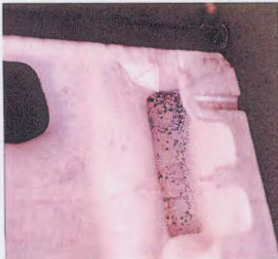
Photo 14. "A" brand Enlarged view of area B Location of most serious corrosion
