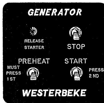
REMOTE START/STOP PANEL
